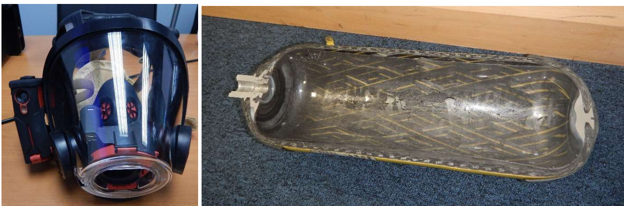
6. Figure: A mask equipped with a thermal camera and an internal monitor and a fully composite compressed-air bottle cut in half. (Photo: Péter Pántya, 2017, 2019)
