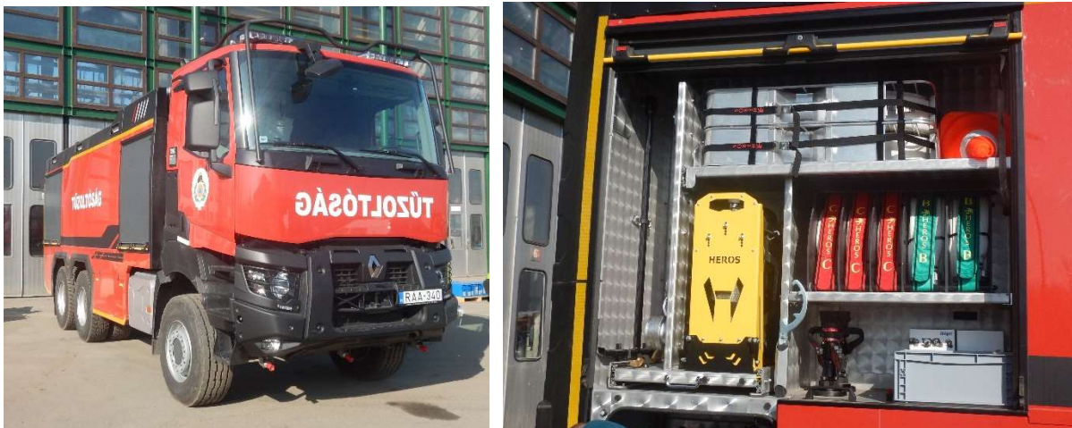
1. Figure: The new Heros Aquarex S10 water carrier in front of the and the placement of the hose packages attached to it in the rear area. (Photo: Péter Pántya, 2019)
