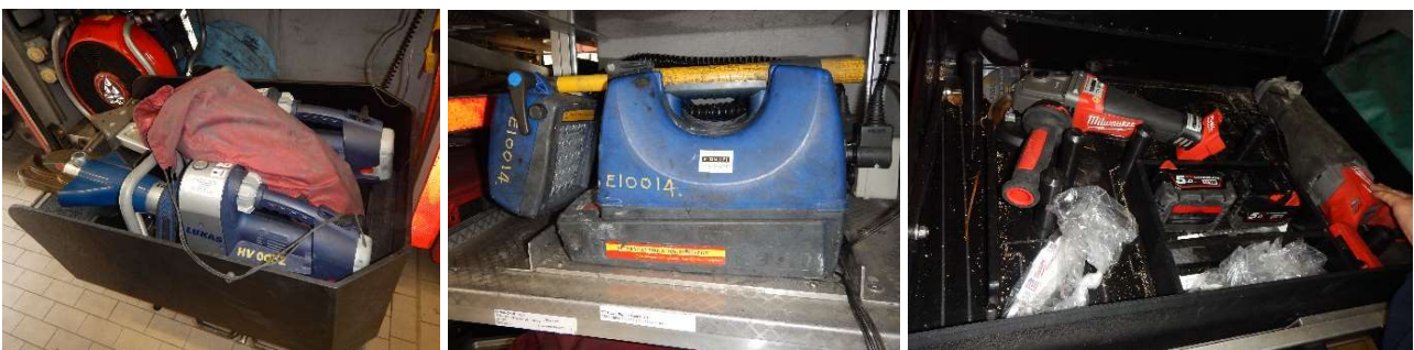
4. Figure: Battery-operated electric tools (hydraulic rescue equipment, mobile damage site lighting and hand-held small machines) on a fire engine in England. (Photo: Péter Pántya, 2017)
