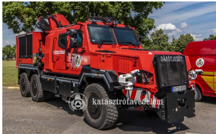
3. Figure: The Komondor, RDO 4336 MPV multi-purpose firefighting vehicle with technical rescue replacement superstructure (Source: Hungarian Disaster Management, 2020, edited by the author)
