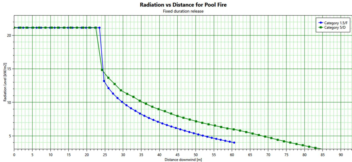
6. Figure: Heat radiation and distance, without remediation board. Prepared by the authors.
